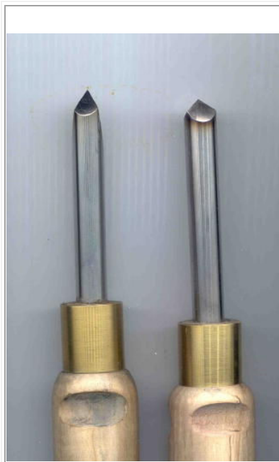
A standard Pyramid Point Tool on the right with a modified Shear Spear Pyramid Point Tool on the left.
