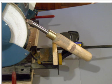
Sharpening the Primary Bevel of a Shear Spear on a Bench Grinder.
