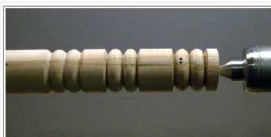
A comparison of beads. On the left are two beads turned with a standard Pyramid Point Tool. In the middle are two beads turned with a Shear Spear. On the right are two beads turned with a Skew.
