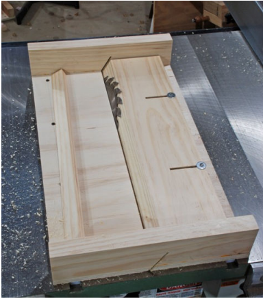
Fig09 The fence after beveling.
