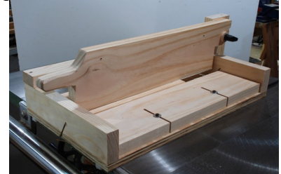
Fig16 Set-up to rip triangles.
