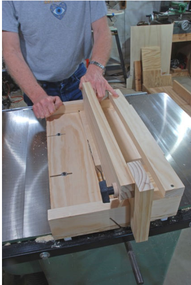
Fig18 Ripping triangles with the rip sled.
