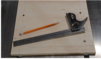
Fig03 Using a square to lay out the position of the front.
