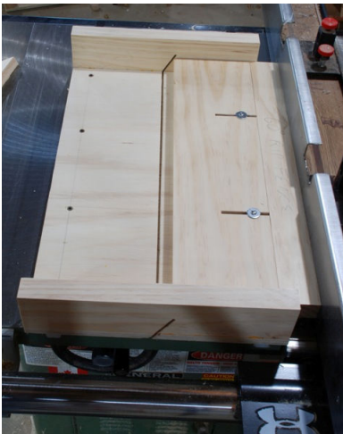
Fig10 The fence after flipping it over so that the bevel faces down.
