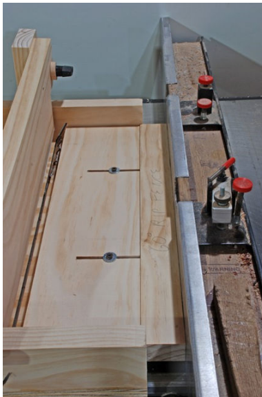
Fig15 Using the fence extension, and table saw fence to set the fence.
