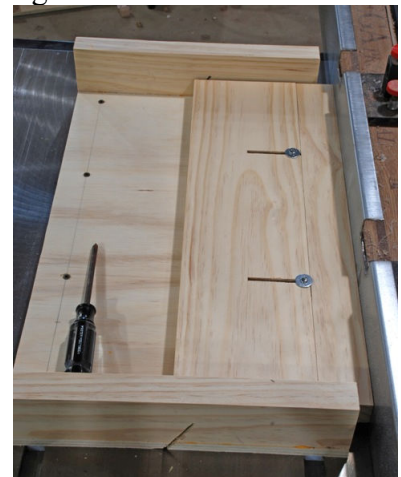
Fig08 Aligning the fence with the right edge of the blade kerf to bevel the fence. The fence extension and your table saw fence make it easier to get the fence parallel to the blade.
