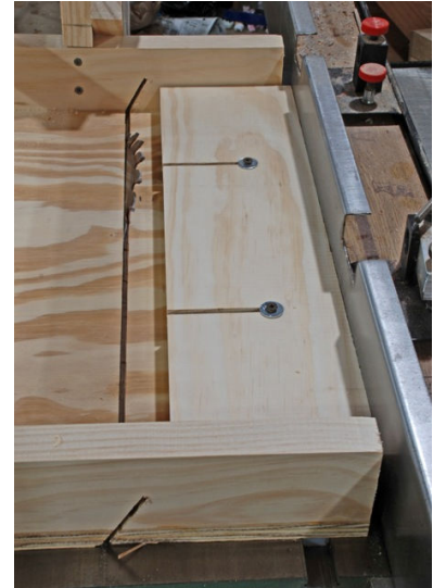
Fig20 After reversing the fence so the 90 degree edge faces the blade.
