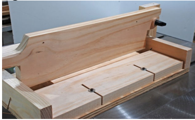
Fig14 Adjusting the hold down height.
