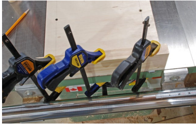
Fig04 Clamping the front to the base.
