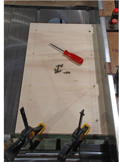
Fig02 Mounting the miter gauge running strips.
