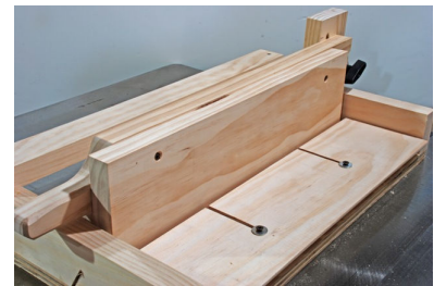
Fig21 After attaching the auxiliary fence.
