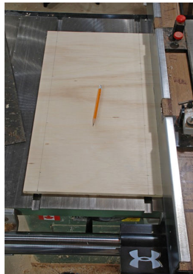
Fig01 Laying out mounting holes for the miter gauge runners.
