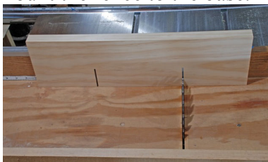
Fig07 Using the table saw to cut slots in the fence.
