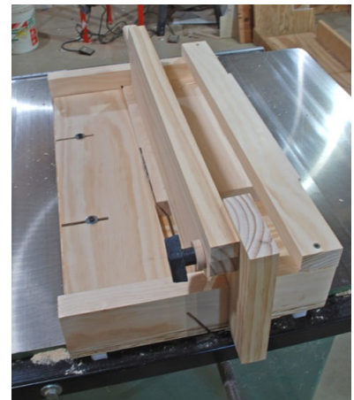
Fig 17 Set-up to rip triangles from the back.
