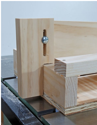
Fig13 After mounting the hold down on the support.
