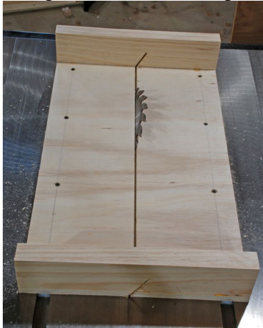
Fig06 Cutting the blade slot with the blade set at 60 degrees.
