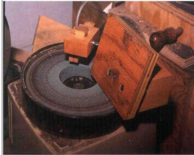
This photo shows the scraper rest mounted on the Makita. The rest is mounted so that the grinding wheel turns away from the edge.
