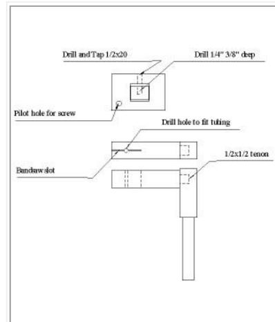
A drawing of the parts for the Water Handler.
