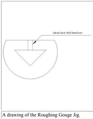
A drawing of the Roughing Gouge Jig.
