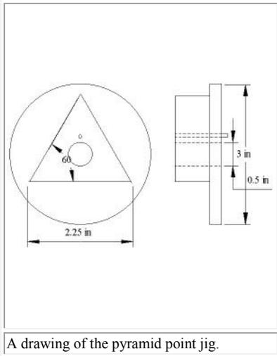
A drawing of the pyramid point jig.
