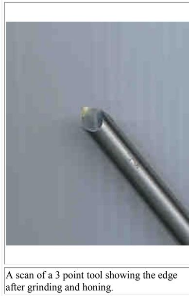
A scan of a 3 point tool showing the edge after grinding and honing.
