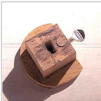
This photo shows the jig for sharpening diamond cross-section parting tools.
