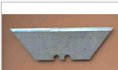
A common utility knife blade. The left hand side has been honed on the honing disk about 15 seconds or so. The difference is more striking in real life.
