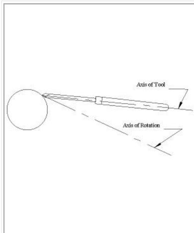
This drawing shows the relationship of the gouge axis to the axis of rotation.
