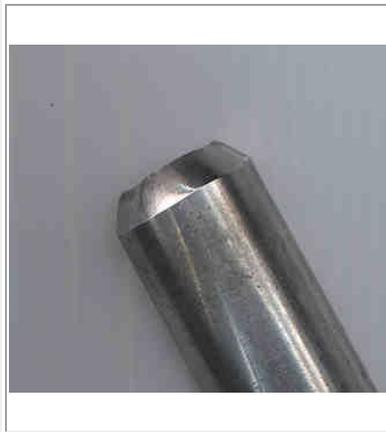
A scan of my Roughing Gouge after grinding and honing. I've also polished the first few inches of the tool on the honing disk so that it slides easier on tool rest.
