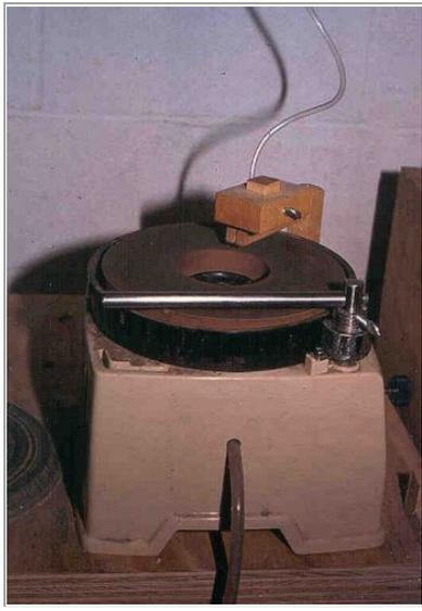
This photo shows the Makita set up to grind with the fine stone, with the adjustable Straight Line Reference and water handling system.
