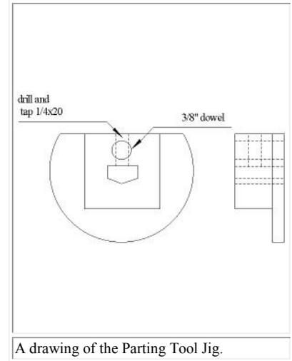
A drawing of the Parting Tool Jig.
