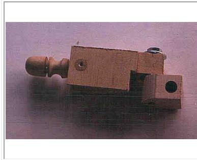
This photo shows the jig that can be used with any gouge if it's used with a stop block to measure the gouge projection. I'm using a homemade handle on all-thread because a long thread is needed depending on the gouge.
