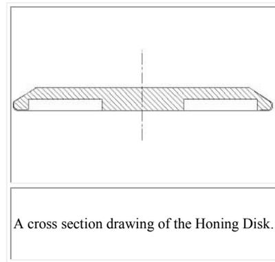
A cross section drawing of the Honing Disk.
