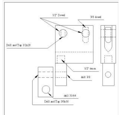
A drawing of the Gouge AutoLength Jig for large gouges.
