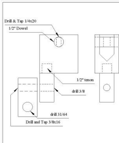
A drawing of the measured length gouge jig.
