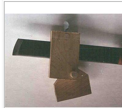
The Curved Skew Jig with the skew mounted. Note that the long point side is next to the pivot.
