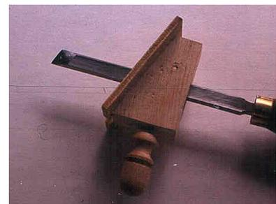
A photo of the skew jig with a skew mounted. Note that the edge of the skew matched the front
