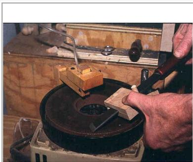
This photo shows sharpening a curved skew. My left hand is squeezing the two parts of the jig together as my right hand rotates the assembly and lifts to apply pressure.
