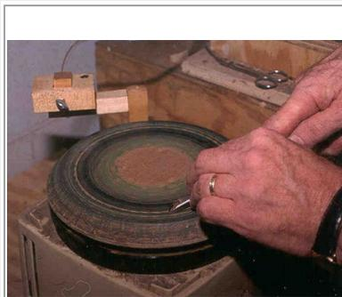
This photo shows honing a skew. The disk is turning away from the edge, and as good contact is made I've increased pressure.
