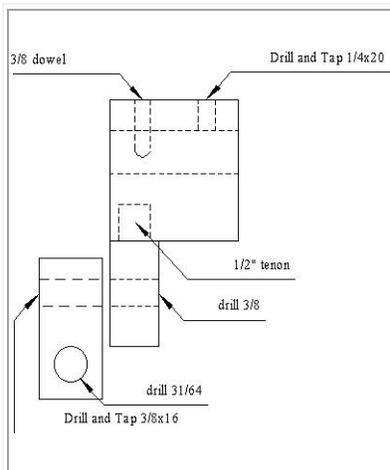
A drawing of the Gouge AutoLength for small gouges.
