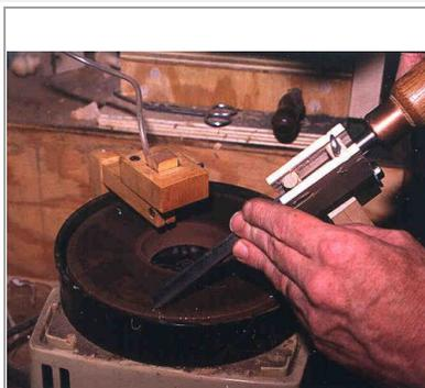
This photo shows sharpening my half inch spindle gouge.
