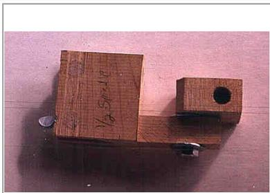
This is the jig I use for my half inch spindle gouge. You may notice that the pivot is at the other end of the block from the drawing. It doesn't really matter as long as you
