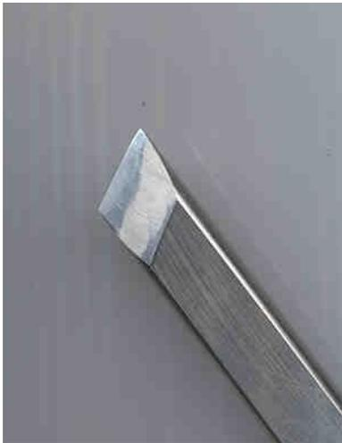
This is a scan of my 1/2" rolled edge skew after sharpening and honing.
