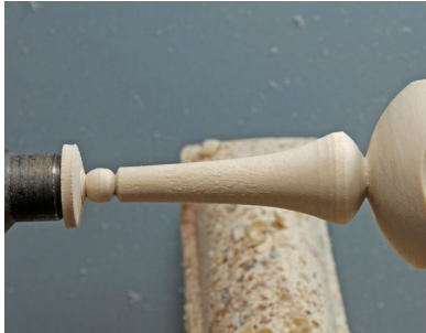
Fig28: After turning the ball at the end of the bottom finial.
