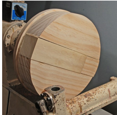
Fig11: The jig with an ornament blank mounted. As the blank is completely encased by the filler pieces there is no propeller effect.
