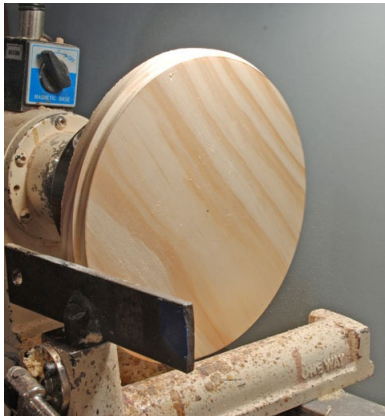
Fig04: After mounting the backplate via the tenon disc in the chuck and turning the front half of the backplate rim to 8" diameter.
