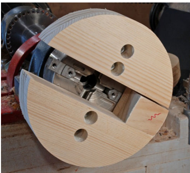
Fig10: An alternate jig using wooden jaws you could use instead if you are comfortable with wooden jaws and have a large 4-jaw chuck.
