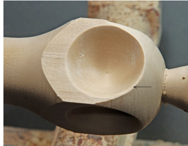
Fig23: After almost rounding over the top half of the globe. Check all four hollows for flat spots such as indicated by the arrow.
