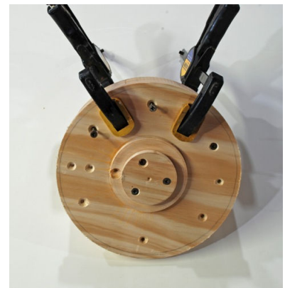
Fig08: Attaching the filler pieces. Clamps hold the filler piece in position while screws are driven in.
