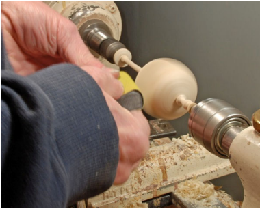
Fig30: Sanding the globe with abrasive wrapped around a foam block.
