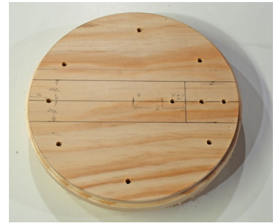
Fig07: Holes for mounting screws for the filler pieces have been drilled in the backplate.
