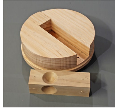
Fig18: The jig and ornament blank after turning all four hollows.
