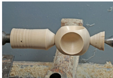
Fig24: The rounding of the globe is complete.
