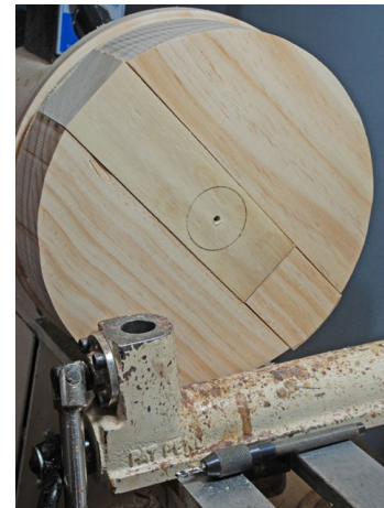
Fig13: After drilling a depth indicator hole. The pin chuck laying on the lathe bed has a drill protruding the right amount.
