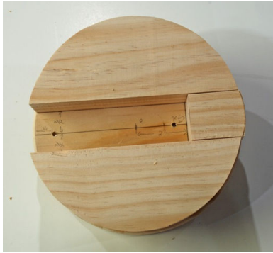
Fig09: The completed jig. The ornament blank is held in between the filler pieces by wood screws in wood that will be turned away later.
