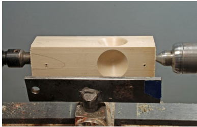
Fig20: The ornament blank mounted between centers.
