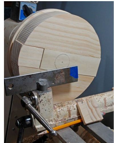
Fig12: After marking the rotation axis and maximum diameter of the hollow. The simple gauge to mark the diameter is leaning on my tool rest banjo.
