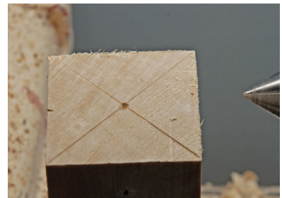
Fig19: After carefully marking and center punching the centers of the ornament blank. Centering must be accurate for the hollows to look the same size.
