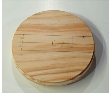
Fig05: After laying out the positions of the filler pieces on the backplate.
