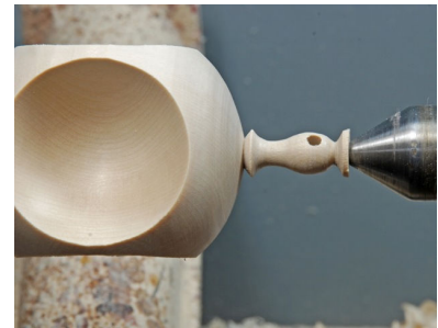
Fig26: The top finial is complete except for a nub for the tailstock.
