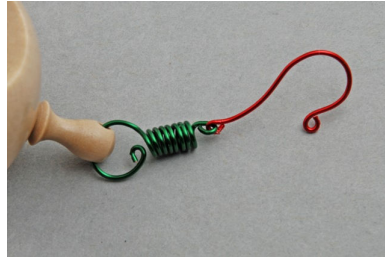
Fig37: After inserting the hanger in the mounting hole and forming a loop so it can't come out.
