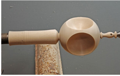
Fig27: After reducing the bottom finial to its largest diameter.
