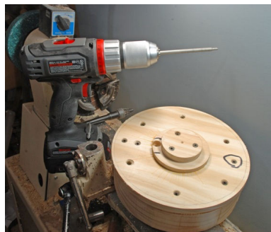
Fig17: Rotating the ornament blank in the jig. I'm using square drive screws which power drive well. The mounting holes are circled with marker to avoid removing the wrong screws.
