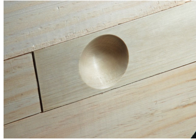
Fig16: After sanding the hollow. If you wish to apply finish on the lathe you should finish the hollow at this point.
