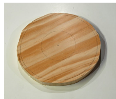
Fig02: The backplate after roughing out on the bandsaw. The diameter of the tenon disc is marked in the center.
