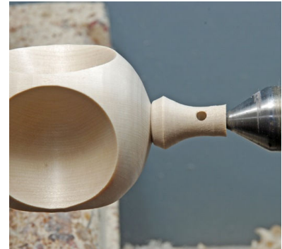
Fig25: After drilling a mounting hole.
