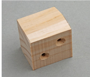
Fig06: After drilling mounting holes in the stop block.
