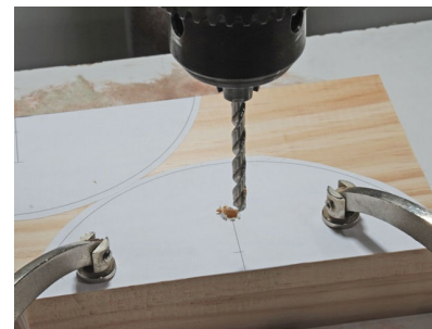
Fig02: Drilling holes for the mounting screws in the wooden jaws.
