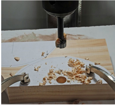
Fig03: Drilling a recess in the wooden jaws for the washers and mounting screws.
