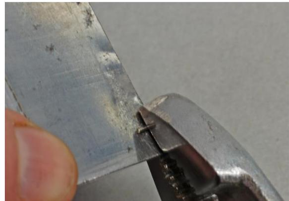
*Fig06: Bend wire around cabinet scraper.*
