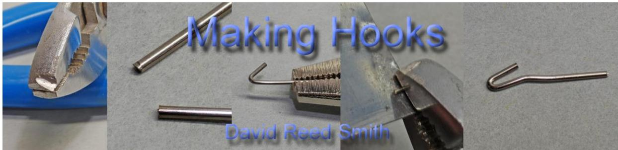
To make hooks for drop spindles I start with 0.043" diameter stainless steel music wire. Anything around this size should work fine.
