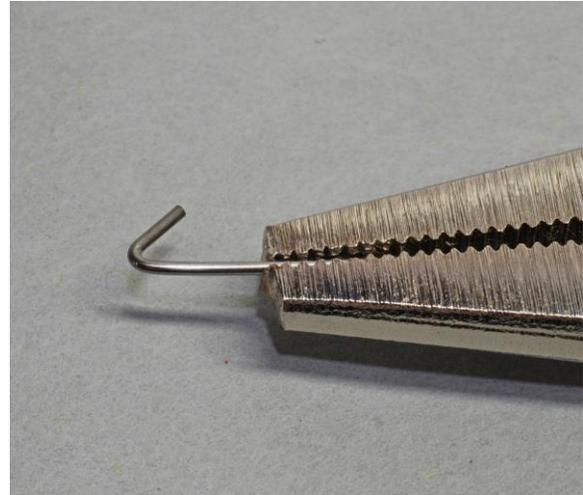
*Fig05: Bend end with modified pliers.*
