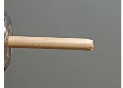
Fig05: Beveling the dowel end to make it easier to start the sizing plate.
