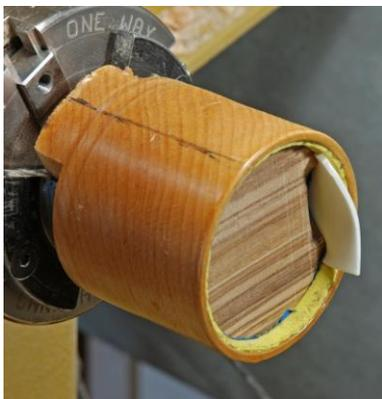
Fig02: Using craft foam to get a vacuum seal around the mouth.
