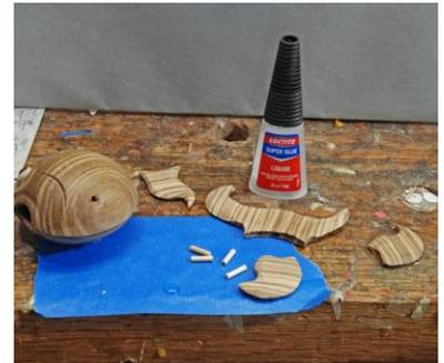
Fig23: The set-up for inserting dowels into fins.
