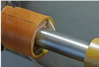
Fig01: Aligning the half blank in the sphere chuck using the tailstock ram.
