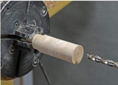
Fig10: Drilling for the eccentric pupil.
