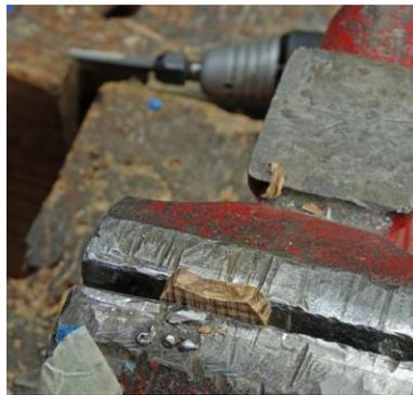
Fig21: After carving a shallow concave groove.
