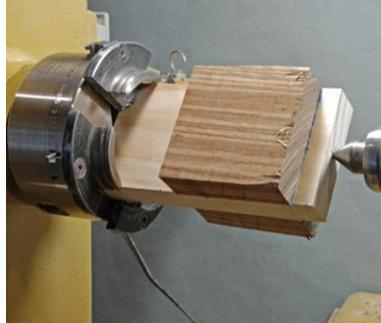
Fig03: Using a longer waste block and the sides of the jaws to automatically center the waste block.
