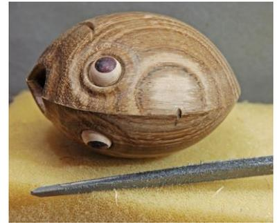
Fig22: Notching the fish to make it easier to start the dowel drill with an awl.
