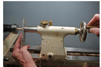
Fig06: Sizing the dowel by advancing the drill sizing plate perpendicularly down the dowel.
