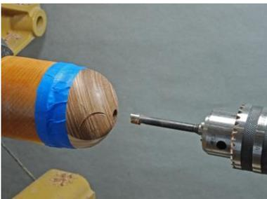
Fig11: Drilling the eye socket.
