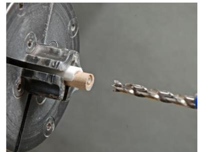
Fig07: Drilling an eccentric pupil hole using a shim and a 4-jawed chuck.
