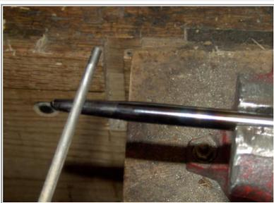
Testing for hardness with a file.
