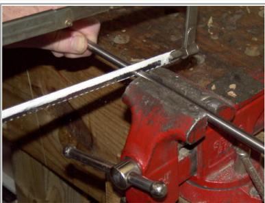
Cutting the Oil Hardening Drill Rod to length with a hacksaw.
