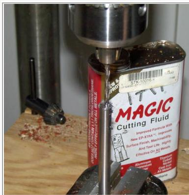
Drilling the end of the Drill Rod to shape the flute.
