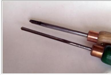
A comparison of the store bought and homemade gouges.
