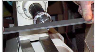
Filing a taper on the Drill Rod while the lathe is turning slowly.
